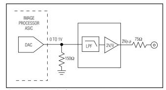
Figure 3. The video DAC generates a 1V<sub>P-P</sub> signal across a  $150\Omega$  resistor connected to ground.
