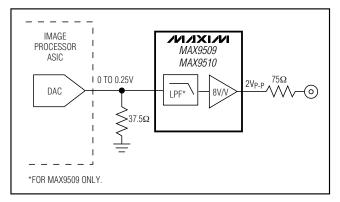
Figure 4. The video DAC generates a 0.25Vp-p signal across a  $37.5\Omega$  resistor connected to ground.
