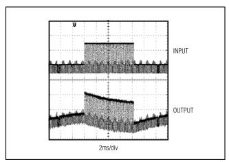
Figure 1. AC-Coupled Output
