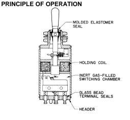
A holding coil in ET toggle switches replaces mechanical holding mechanisms to maintain the toggle in an operate position. The toggle is released by breaking the coil circuit.
