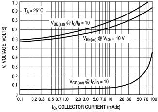
Figure 2. "Saturation" and "On" Voltages
