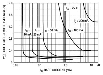
Figure 3. Collector Saturation Region
