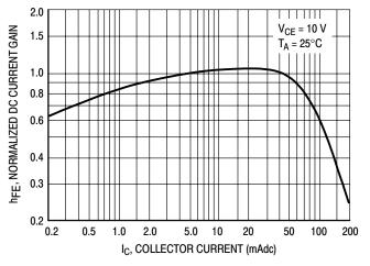
Figure 1. Normalized DC Current Gain
