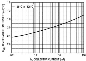
Figure 4. Base-Emitter Temperature Coefficient
