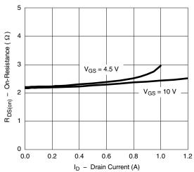
On-Resistance vs. Drain Current
