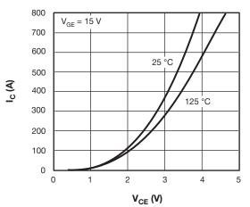
Fig. 1 - IGBT Typical Output Characteristics
