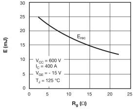
Fig. 9 - Diode Switching Loss vs.Rg
