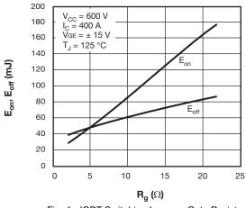
Fig. 4 - IGBT Switching Loss vs. Gate Resistor
