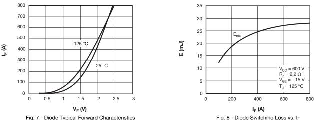
Fig. 8 - Diode Switching Loss vs. IF
