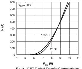
Fig. 2 - IGBT Typical Transfer Characteristics
