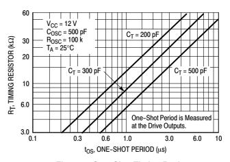
Figure 5. One-Shot Timing Resistor versus Period
