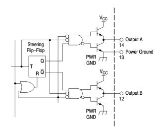
Figure 18. Steering Flip-Flop and Output Drivers
