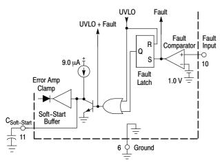
Figure 20. Fault Detector and Soft-Start
