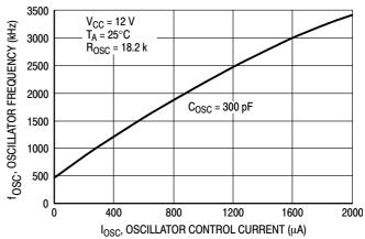
Figure 3. Oscillator Frequency versus
