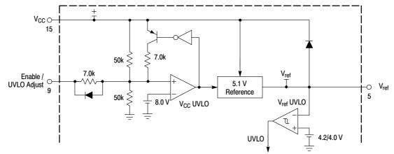
Figure 19. Undervoltage Lockout and Reference
