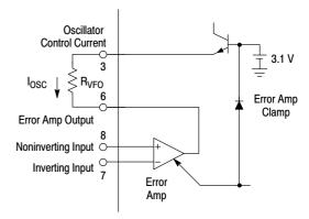
Figure 17. Error Amplifier and Clamp
