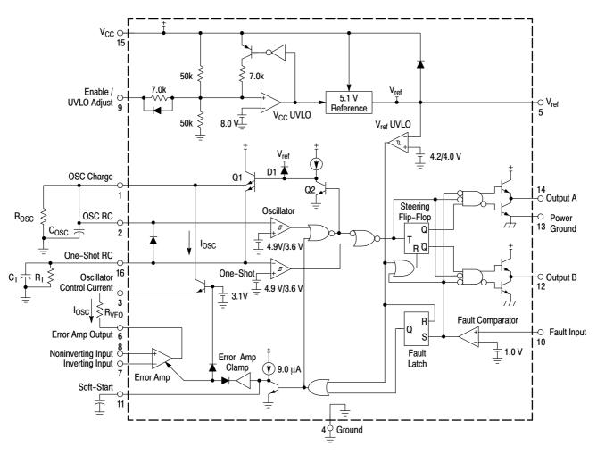
Figure 14. MC34067 Representative Block Diagram
