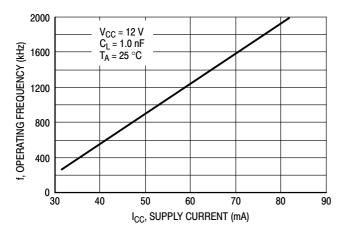
Figure 12. Operating Frequency versus Supply Current
