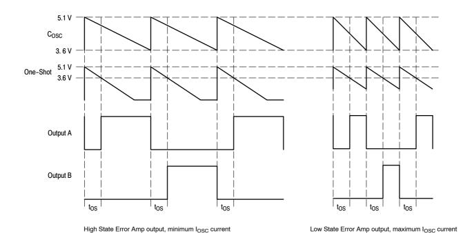
Figure 15. Timing Diagram
