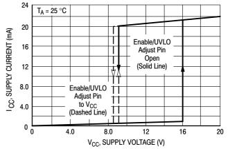
Figure 13. Supply Current versus Supply Voltage
