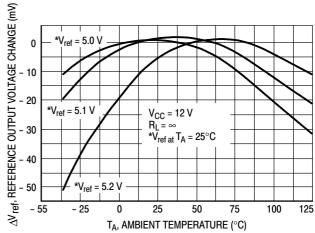
Figure 7. Reference Output Voltage Change versus Temperature
