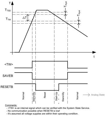
Figure 8. Temperature Monitoring Levels
