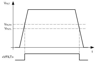
Comments: <VFILT> is an internal signal which can be verified with the System State Service
