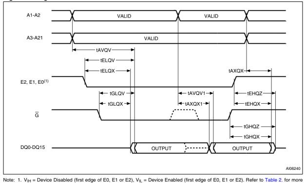
Figure 10. Page Read AC Waveforms
