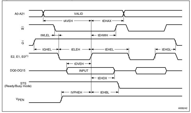
Figure 12. Write AC Waveforms, Chip Enable Controlled
