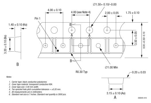
Figure 10. SOT-5 Tape and Reel Dimensions
