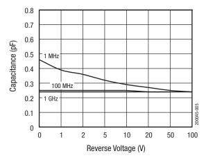
Figure 5. Capacitance vs Reverse Voltage
