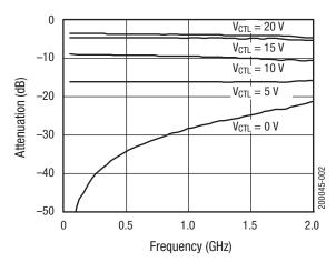
Figure 2. SMP1307-027 Attenuation vs Frequency
