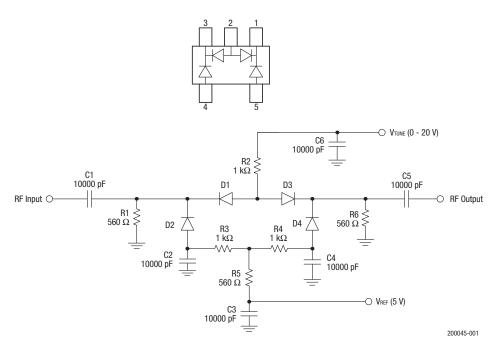
Figure 1. SMP1307-027 Block Diagram and Schematic
