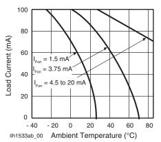
Fig. 1 - Recommended Operating Conditions
