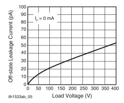
Fig. 5 - Leakage Current vs. Applied Voltage
