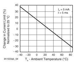
Fig. 4 - Current Limit vs. Temperature
