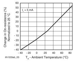
Fig. 3 - On-Resistance vs. Temperature
