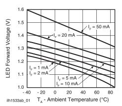
Fig. 2 - LED Voltage vs. Temperature
