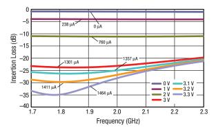
Figure 3. Insertion Loss vs Frequency vs Control Voltage
