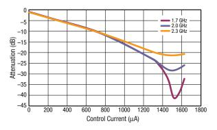
**Figure 6. Attenuation vs Control Current vs Frequency**
