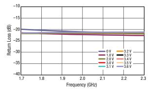
Figure 4. Return Loss vs Frequency vs Control Voltage
