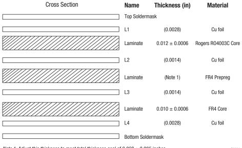
Note 1: Adjust this thickness to meet total thickness goal of 0.062  $\pm$  0.005 inches.
