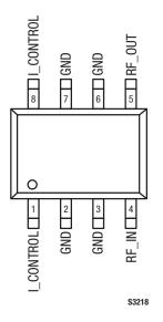
Figure 2. SKY12230-12LF Pinout – 8-Pin SOIC (Top View)
