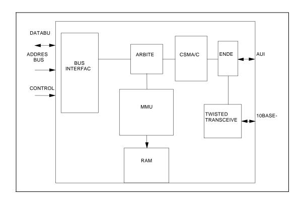
Figure 1 - LAN91C96i Internal Block Diagram
