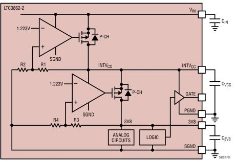
NOTE: PLACE  $C_{VCC}$  and  $C_{3V8}$  capacitors as close as possible to device pins
