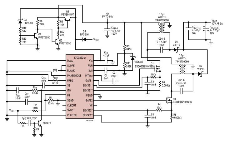
A 6V to 60V Input, 12V/6A Output 2-Phase SEPIC Application Circuit
