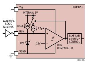
Figure 5b. On/Off Control Using External Logic
