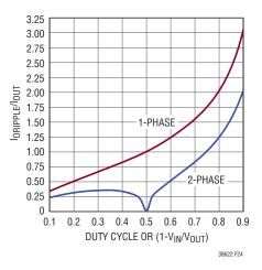
Figure 24. Normalized Output Capacitor Ripple Current (RMS) for a Boost Converter
