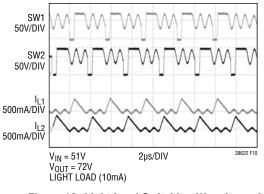
Figure 10. Light Load Switching Waveforms for the LTC3862-2 at the Onset of Pulse-Skipping
