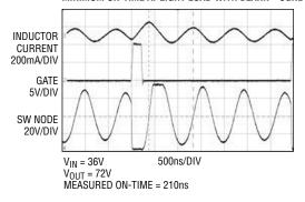
MINIMUM ON-TIME AT LIGHT LOAD WITH BLANK = FLOAT
