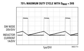
Figure 14. SW Node Waveforms with Different Duty Cycle Limits
