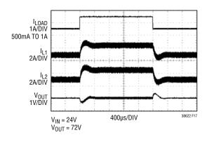
Figure 17. Load Step Response of a Properly Compensated Boost Converter
