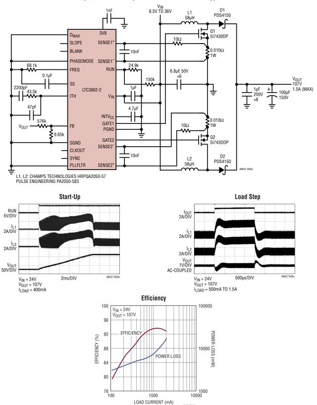
A 24V Input, 107V/1.5A Output 2-Phase Boost Converter Application Circuit
