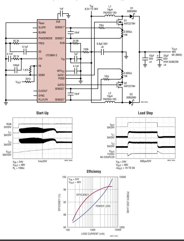
A 24V Input, 48V/6A Output 2-Phase Boost Converter Application Circuit
