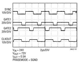
Figure 7. Synchronization of the LTC3862-2 to an External Clock Using the PLL
