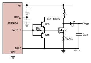
Figure 19. External Buffer Circuit
