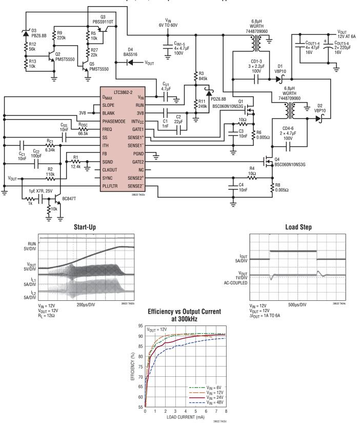
A 6V to 60V Input, 12V/6A Output 2-Phase SEPIC Application Circuit
