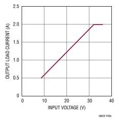
Figure 26b. Output Current vs Input Voltage
