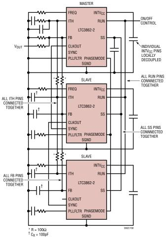
Figure 8. LTC3862-2 Error Amplifier Configuration for Multi-Phase Operation
