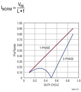
Figure 25. Normalized Input Peak-to-Peak Ripple Current
