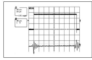
Figure 7. ESD response to IEC 61000-4-2 (-15 kV air discharge) on one imput (V<sub>in</sub>) and one output (V<sub>out</sub>)
