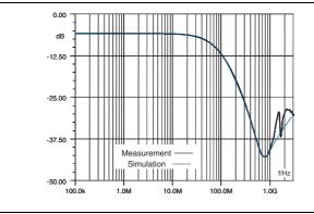
Figure 5. Digital crosstalk measurements
