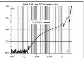
Figure 6. ESD response to IEC 61000-4-2 (+15 kV air discharge) on one imput (V<sub>in</sub>) and one output (V<sub>out</sub>)
