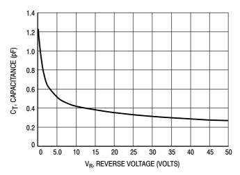
Figure 3. Typical Capacitance
