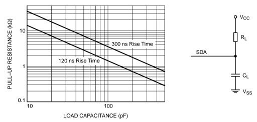
Figure 2. Pull-up Resistance vs. Load Capacitance
