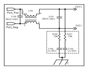
Figure 1: Recommended EMI Filter
