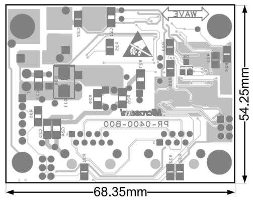
Figure 3: Layout Example of Component and Print Side
