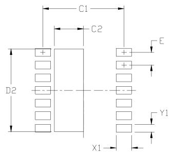
Figure 52. 14-Pin LGA with Thermal Pad Land Pattern
