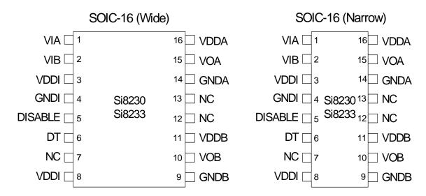
Table 11. Si8230/3 Two-Input HS/LS Isolated Driver (SOIC-16)
