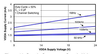
Figure 13. Supply Current vs. Supply Voltage
