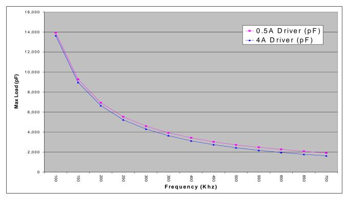
Figure 35. Max Load vs. Switching Frequency
