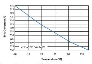
Figure 21. Output Sink Current vs. Temperature
