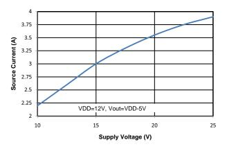
Figure 32. Output Source Current vs. Supply Voltage
