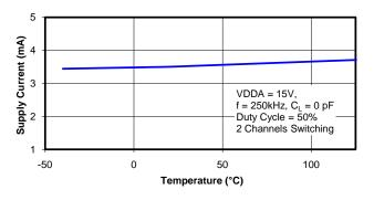
Figure 15. Supply Current vs. Temperature
