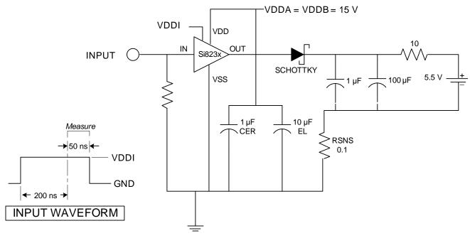
**Figure 5. IOH Source Current Test Circuit**
