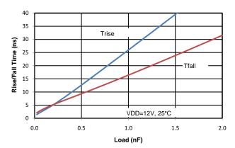
Figure 16. Rise/Fall Time vs. Load
