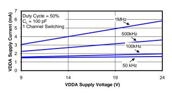
Figure 14. Supply Current vs. Supply Voltage
