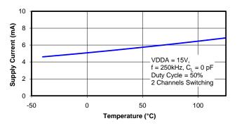
Figure 27. Supply Current vs. Temperature
