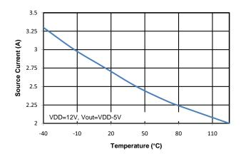
Figure 34. Output Source Current vs. Temperature
