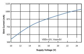
Figure 19. Output Sink Current vs. Supply Voltage
