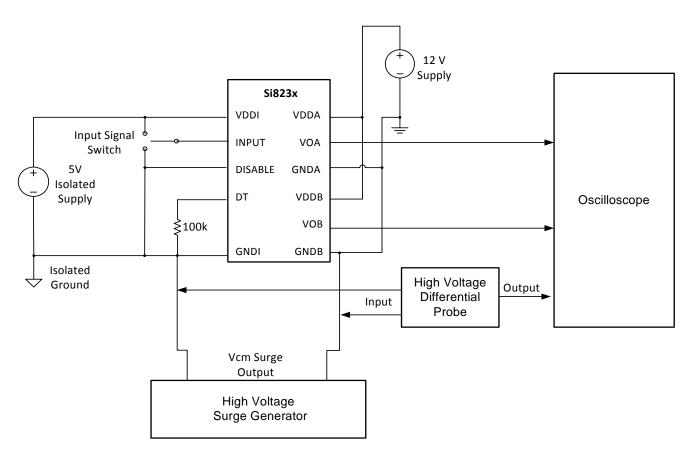
Figure 6. Common Mode Transient Immunity Test Circuit
