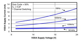
Figure 25. Supply Current vs. Supply Voltage
