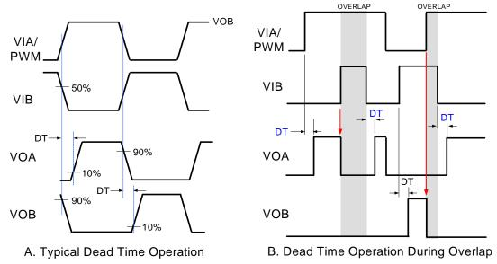
Figure 42. Dead Time Waveforms for High-Side/Low-Side Two-Input Drivers
