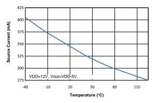
Figure 22. Output Source Current vs. Temperature
