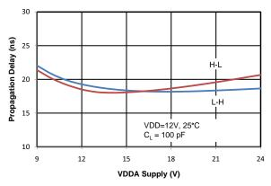
Figure 12. Propagation Delay vs. Supply Voltage
