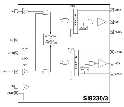
Figure 1. Si8230/3 Two-Input High-Side/Low-Side Isolated Drivers
