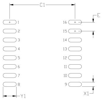
Figure 46. 16-Pin SOIC Land Pattern
