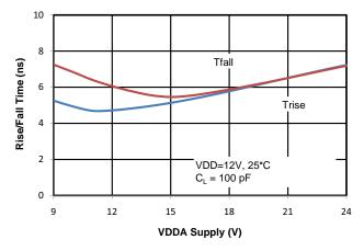
Figure 23. Rise/Fall Time vs. Supply Voltage
