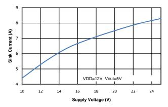
Figure 31. Output Sink Current vs. Supply Voltage
