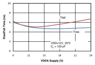
Figure 11. Rise/Fall Time vs. Supply Voltage
