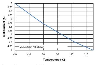
Figure 33. Output Sink Current vs. Temperature
