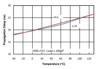
Figure 30. Propagation Delay vs. Temperature
