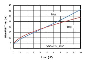
Figure 28. Rise/Fall Time vs. Load
