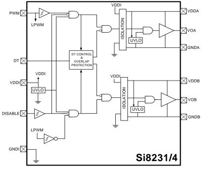
Figure 2. Si8231/4 Single-Input High-Side/Low-Side Isolated Drivers
