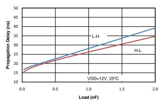
Figure 17. Propagation Delay vs. Load
