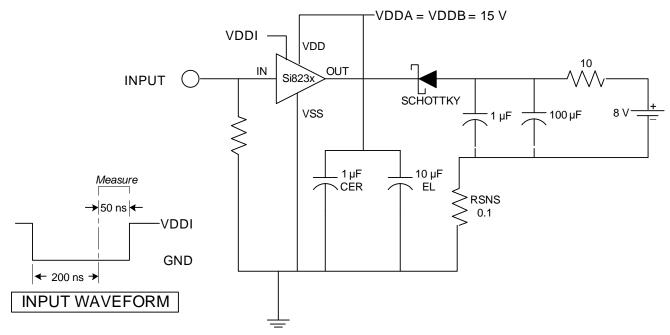
Figure 4. IOL Sink Current Test Circuit
