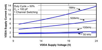
Figure 26. Supply Current vs. Supply Voltage
