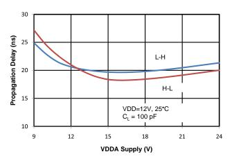
Figure 24. Propagation Delay vs. Supply Voltage
