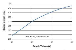
Figure 20. Output Source Current vs. Supply Voltage
