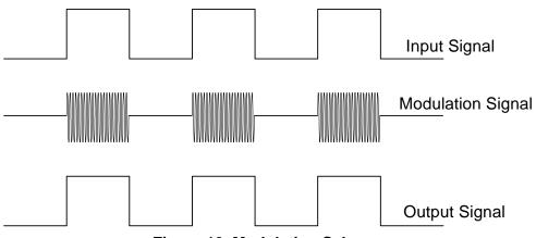
Figure 10. Modulation Scheme
