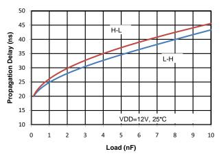
Figure 29. Propagation Delay vs. Load
