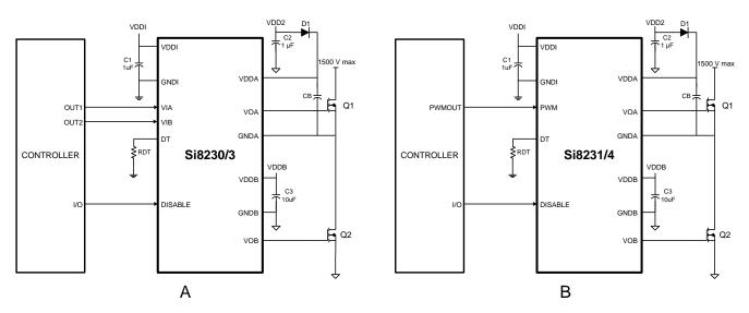
Figure 43. Si823x in Half-Bridge Application
