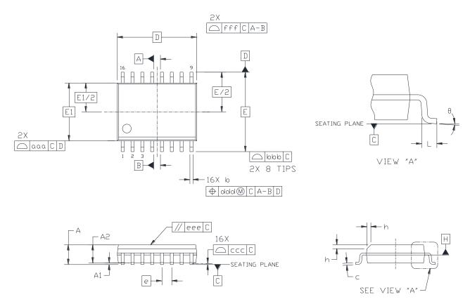
Figure 45. 16-Pin Wide Body SOIC
