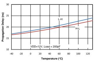
Figure 18. Propagation Delay vs. Temperature
