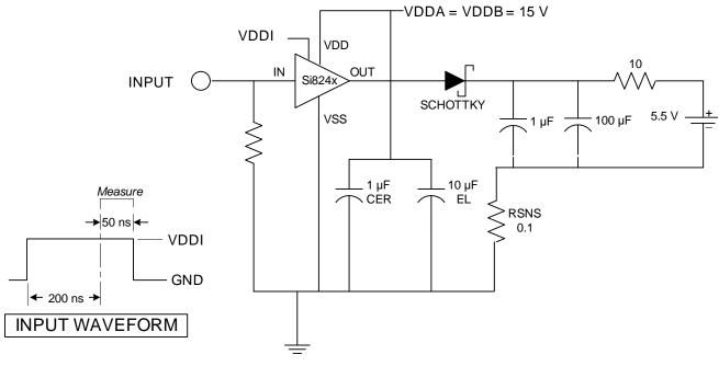
Figure 3. IOH Source Current Test Circuit
