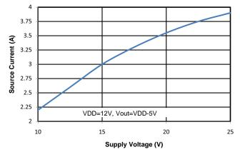
Figure 29. Output Source Current vs. Supply Voltage
