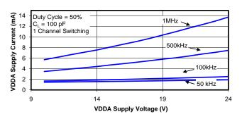
Figure 23. Supply Current vs. Supply Voltage
