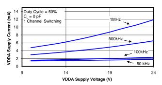
Figure 22. Supply Current vs. Supply Voltage
