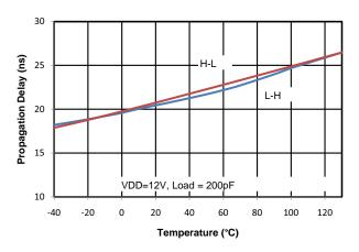
Figure 27. Propagation Delay vs. Temperature
