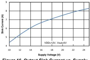
Figure 16. Output Sink Current vs. Supply Voltage
