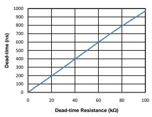
Figure 37. Dead Time vs.Resistance (R<sub>DT</sub>)
