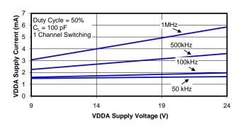
Figure 11. Supply Current vs. Supply Voltage
