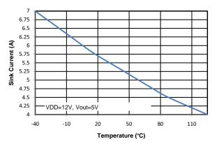
Figure 18. Output Sink Current vs. Temperature
