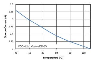
Figure 19. Output Source Current vs. Temperature
