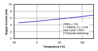
Figure 24. Supply Current vs. Temperature
