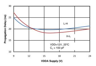
Figure 21. Propagation Delay vs. Supply Voltage
