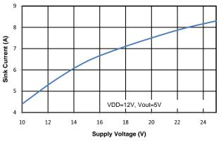
Figure 28. Output Sink Current vs. Supply Voltage
