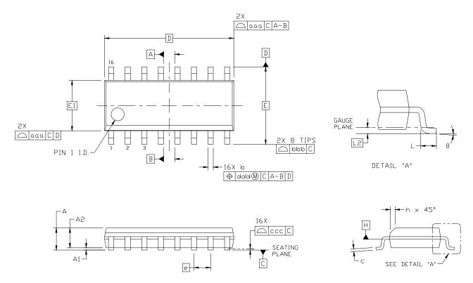
Figure 41. 16-pin Small Outline Integrated Circuit (SOIC) Package
