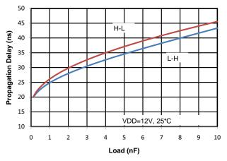
Figure 26. Propagation Delay vs. Load
