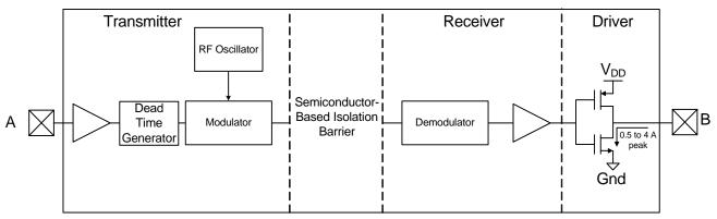
Figure 6. Simplified Channel Diagram
