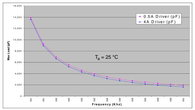
Figure 32. Max Load vs. Switching Frequency
