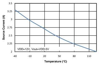
Figure 31. Output Source Current vs. Temperature
