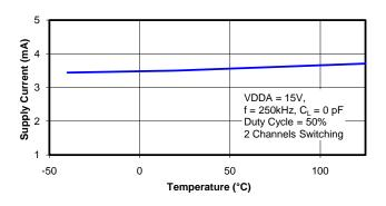
Figure 12. Supply Current vs. Temperature
