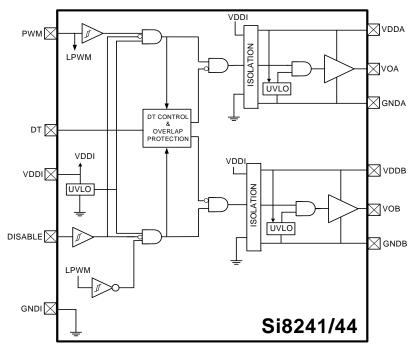
Figure 1. Si8241/44 Single-Input High-Side/Low-Side Isolated Drivers
