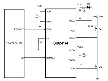
Figure 39. Si824x in Half-Bridge Audio Application
