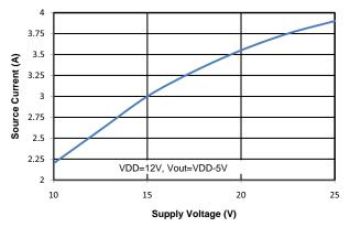
Figure 17. Output Source Current vs. Supply Voltage
