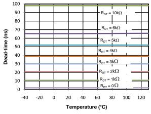
Figure 38. Dead Time vs. Temperature
