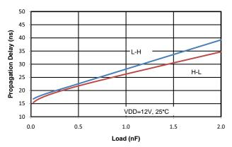
Figure 14. Propagation Delay vs. Load
