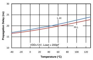
Figure 15. Propagation Delay vs. Temperature
