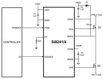
Figure 40. Si824x in Half-Bridge Audio Application
