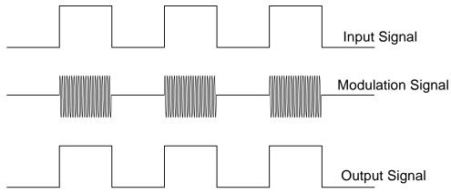
Figure 7. Modulation Scheme
