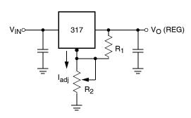
$V_{O}$  (REG) = 1.25V (1 +  $R_2/R_1$ ) +  $I_{adj}$   $R_2$
