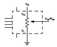
Three terminal potentiometer; variable voltage divider
