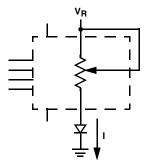
Two terminal variable resistor; variable current
