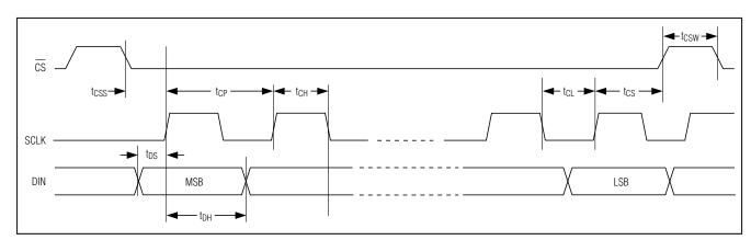
Figure 5. 3-Wire Serial Interface Timing Diagram
