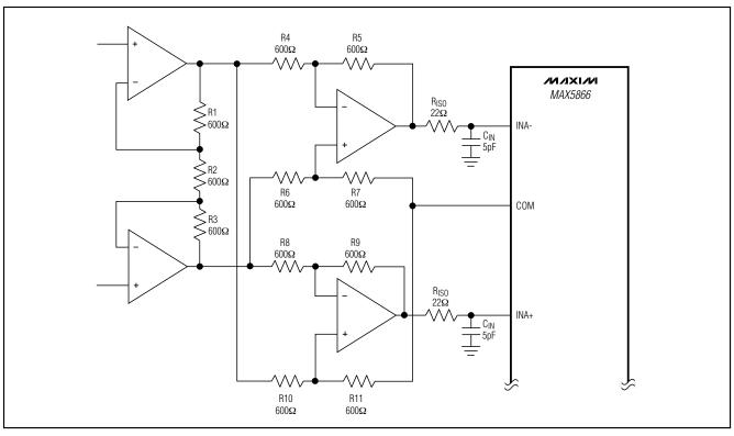
Figure 10. ADC DC-Coupled Differential Drive
