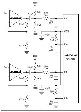
Figure 9. Single-Ended Drive for ADCs
