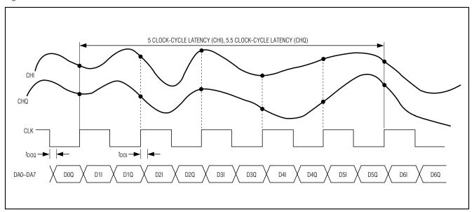
Figure 3. ADC System Timing Diagram
