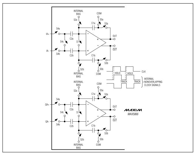
Figure 1. MAX5866 ADC Internal T/H Circuits
