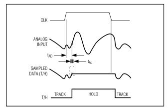
Figure 13. T/H Aperture Timing
