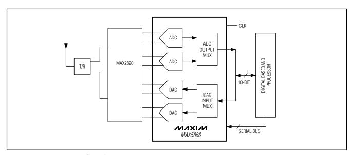
Figure 11. Typical Application Circuit for TDD
