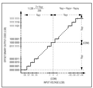
Figure 2. ADC Transfer Function
