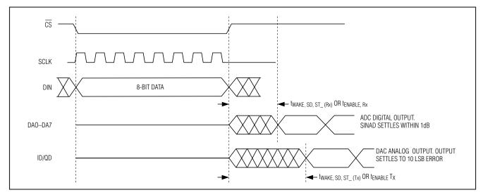
Figure 6. MAX5866 Mode Recovery Timing Diagram
