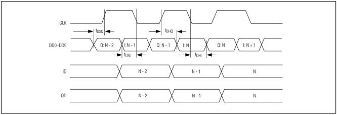
Figure 4. DAC System Timing Diagram
