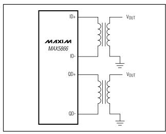
Figure 8. Balun-Transformer-Coupled Differential-to-Single-Ended Output Drive for DACs
