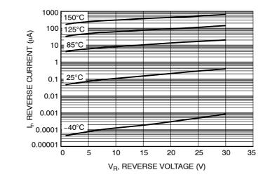
Figure 3. Leakage Current
