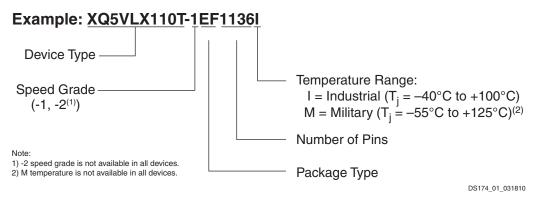
Figure 1: Virtex-5Q FPGA Ordering Information
