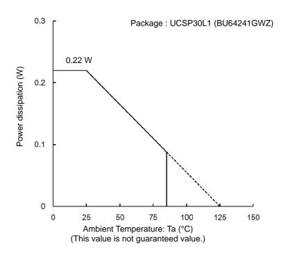
Figure 13. Power dissipation Pd (W)
