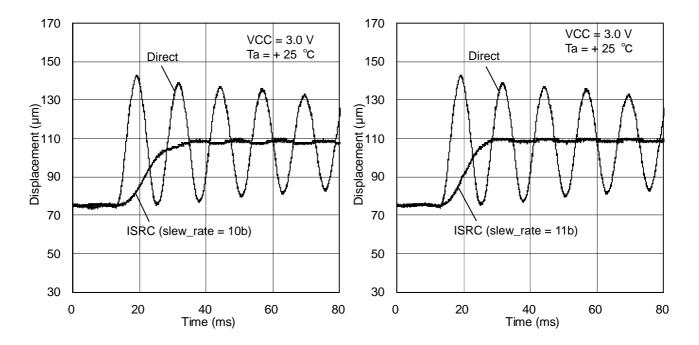
Figure 8. Displacement vs. settling time (slew\_rate = 10b)
