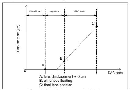
Figure 15. Lens Displacement vs. DAC Code
