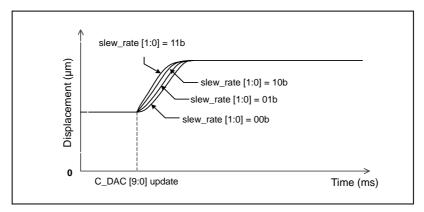
Figure 18. Displacement vs. Settling Time
