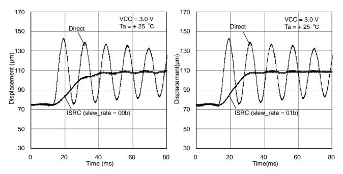
Figure 6. Displacement vs. settling time (slew\_rate = 00b)
