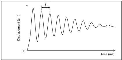
Figure 14. Actuator Displacement Waveform (ISRC Disabled)
