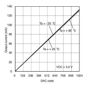
Figure 5. Output current vs. DAC code
