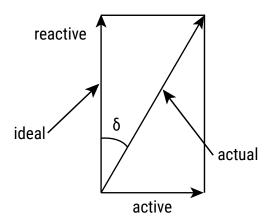
Tan  $\delta$  is measured with the same set-up used for the series capacitance ESC.  $\tan \delta = \omega \times ESC \times ESR$  where:
