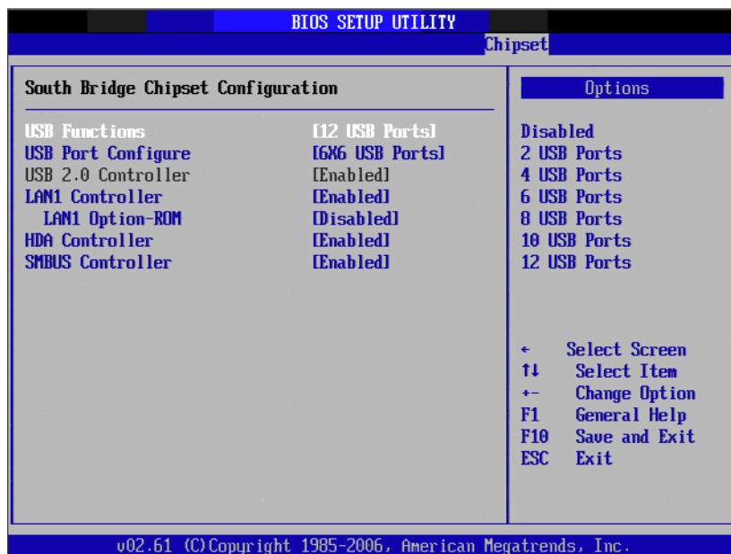
Figure 2.25 South Bridge Configuration
