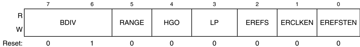
Figure 11-8. ICS Control Register 2 (ICSC2)
