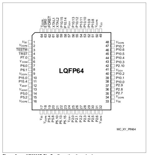
Figure 3 XC2336B Pin Configuration (top view)
