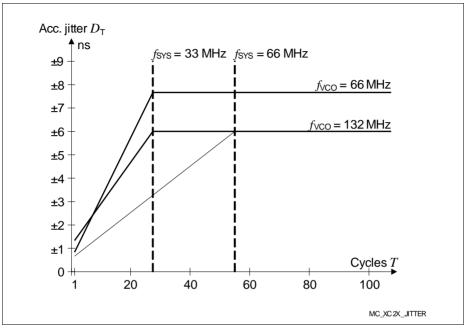
Figure 20 Approximated Accumulated PLL Jitter
