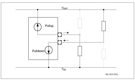
Figure 13 Pullup/Pulldown Current Definition
