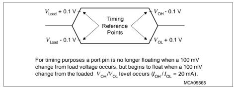
Figure 18 Floating Waveforms
