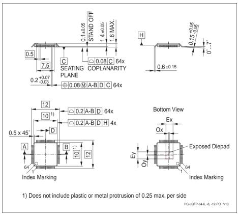
Figure 28 PG-LQFP-64-6/-24 (Plastic Green Thin Quad Flat Package)
