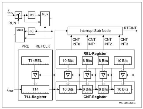
Figure 10 RTC Block Diagram
