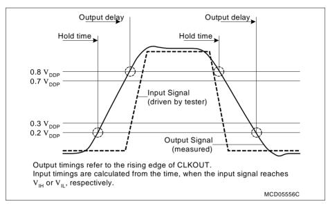
Figure 17 Input Output Waveforms
