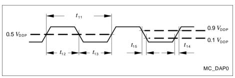
Figure 23 Test Clock Timing (DAP0)
