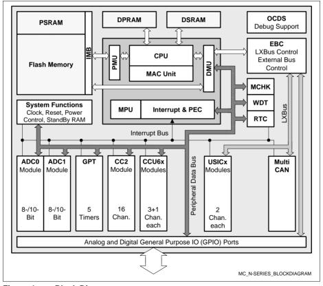
Figure 4 Block Diagram
