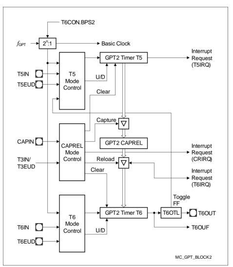
Figure 9 Block Diagram of GPT2
