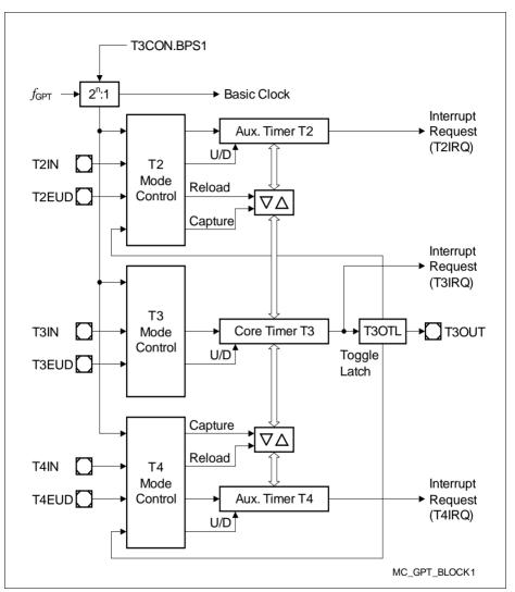
Figure 8 Block Diagram of GPT1
