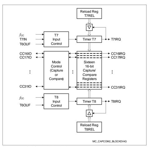
Figure 6 CAPCOM Unit Block Diagram
