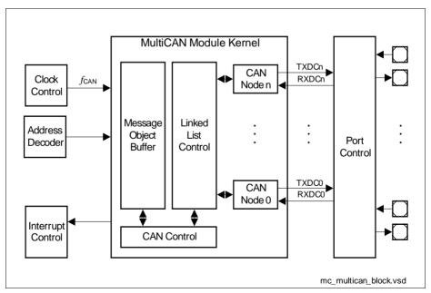
Figure 12 Block Diagram of MultiCAN Module
