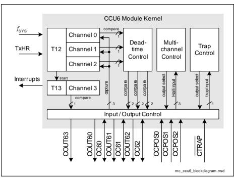
Figure 7 CCU6 Block Diagram
