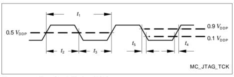
Figure 26 Test Clock Timing (TCK)
