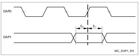
Figure 24 DAP Timing Host to Device
