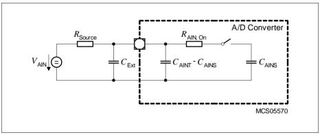
Figure 16 Equivalent Circuitry for Analog Inputs
