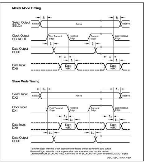
Figure 22 USIC - SSC Master/Slave Mode Timing
