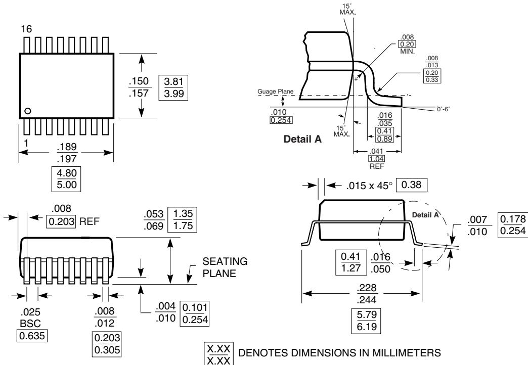
**Packaging Mechanical: 16-Pin SOIC (W)**
