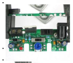
Next we will solder in the 2-pin terminal jack. This lets us connect up wires to power the board from a battery or similar.
