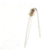
We're going to solder one of the 1.0K resistors in next. The resistors should be bent over 180 like shown. Note that resistors are 'non-polarized' so you can put them in 'either way' - they work the same forwards or backwards.
