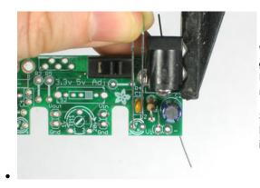
We will finish up the 'high voltage' power supply side by placing the green indicator LED. This LED will let us know that power is working! LEDs are diodes so they are polarized. If not placed correctly they will not work! So make sure you get this right.
