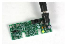
Lets take a break and test the current progress. Take the kit out of the vise and make sure there are no stray wires kicking around that could cause the board to short.
