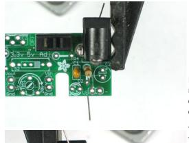
Place one of the 1.0K resistors (Brown Black Red Gold) into the slot marked R1. Then place right next to it one of the 0.1uF ceramic capacitors (they're small and yellow). The resistors and ceramic capacitors are non-polarized so they can go in 'either way'.
