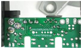
Solder and clip the three resistors.
