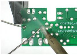
Now solder both wires to the PCB.
