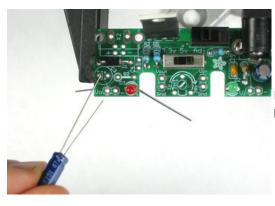
Next is the large electrolytic capacitor. Just like the other one, its polarized. Make sure the long lead goes into the (+) marked pad.
