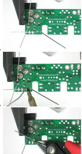
Bend the leads out so the parts sit flat against the PCB.
