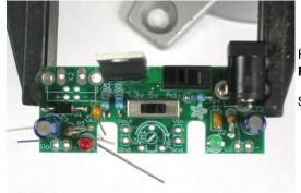
Finish off the 'low voltage' side by inserting the second 1.0K resistor **R2** and the second 0.1uF ceramic capacitor **C4**.
