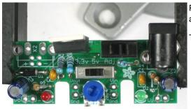
Place the 100K trim potentiometer in the middle. This is what lets us adjust the voltage output from 1.25V to 20V.
