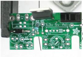
The regulator uses resistors to set the adjustable output voltages. We'll now solder those in.
