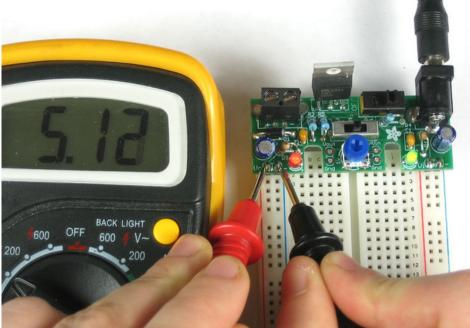
Finally, by selecting **Adj.** you can adjust the supply to anything you want from as low as ~1.3V to within half a volt of the input (which can be as high as 20V).
