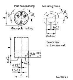
Standard snap-in terminals: length (6.3 + 1/-1.4) mm. Also available with length of (4.5 -1.4) mm. PET insulation cap is positioned under the insulation sleeve.
