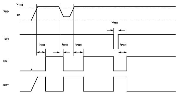
FIGURE 1. POWER-SUPPLY MONITORING TIMING DIAGRAM (WDI TRI-STATED)
