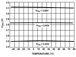
FIGURE 8. V<sub>TH1</sub> vs TEMPERATURE < 5V SUPPLY
