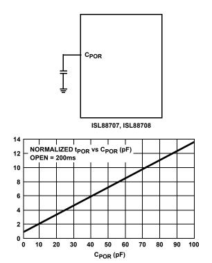
FIGURE 3. ADJUSTING tPOR WITH A CAPACITOR
