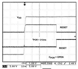
FIGURE 10. RESET AND RESET ASSERTION
