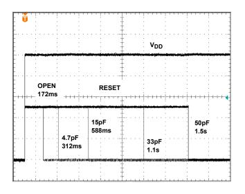
FIGURE 11. RESET ASSERTION vs CPOR
