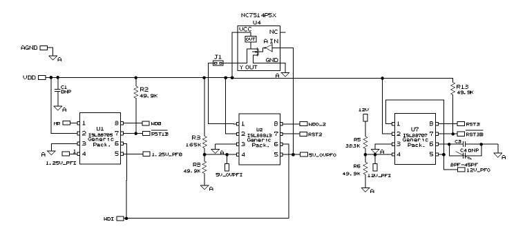
FIGURE 17. ISL88705EVAL1 SCHEMATIC (TOP BANK)
