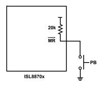
FIGURE 4. CONNECTING A MANUAL RESET PUSH-BUTTON
