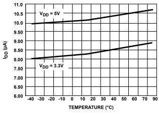
FIGURE 6. I<sub>DD</sub> vs TEMPERATURE
