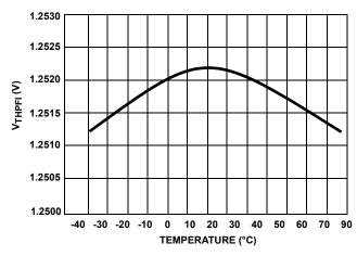
FIGURE 9. V<sub>THPFI</sub> vs TEMPERATURE
