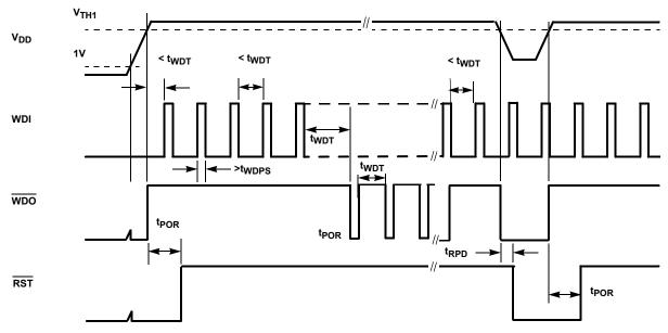
FIGURE 5. WATCHDOG TIMING DIAGRAM
