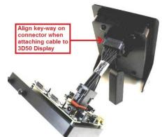
5. Mount the frame with the 3D50 Display to the Breakout Board.
