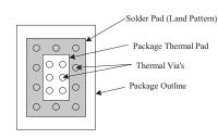
Package and PCB Land Configuration For a Multi-Layer PCB
