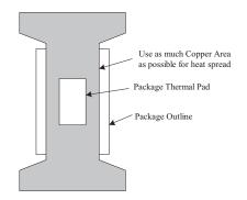
Layout recommendations for a Single Layer PCB: utilize as much Copper Area for Power Management. In a single layer board application the thermal pad is attached to a heat spreader (copper areas) by using low thermal impedance attachment method (solder paste or thermal conductive epoxy).
