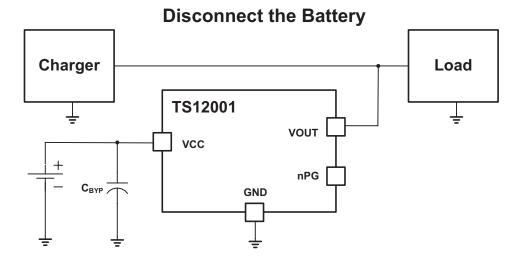
Note: When the TS12001 is Off-Active<sup>™</sup>, the battery will continue to charge through the body diode between VOUT and VCC.
