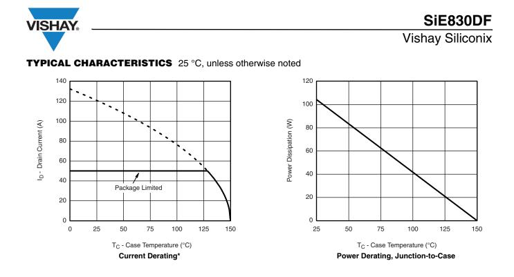
\* The power dissipation  $P_D$  is based on  $T_{J(max)} = 150$  °C, using junction-to-case thermal resistance, and is more useful in settling the upper dissipation limit for cases where additional heatsinking is used. It is used to determine the current rating, when this rating falls below the package limit.
