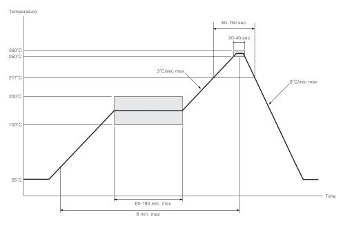
Figure 2-6: Standard Eutectic Solder Reflow Profile
