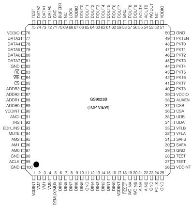
NOTE: The GS9023B DOUT[9:0] MSB to LSB convention is compatible with the GS9022 but reversed with the GS9032 or GS7005. See Interconnection with GS9032 or GS7005 section.
