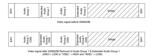
Figure 3-13: Removal of Audio Group 1 with Extended Audio, ADEL=LOW
