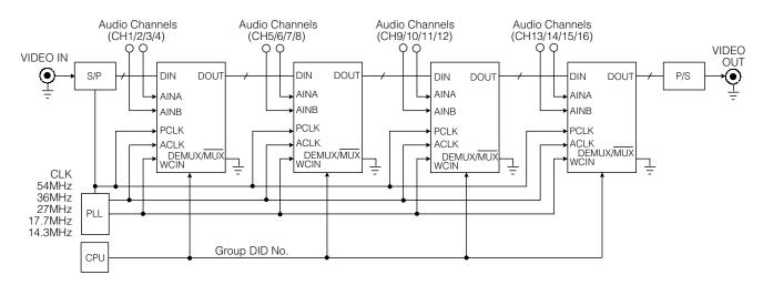
Figure 3-5: Multiplex Mode Cascadable Architecture
