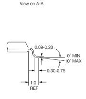
100 pin TQFP Dimensions in millimetres
