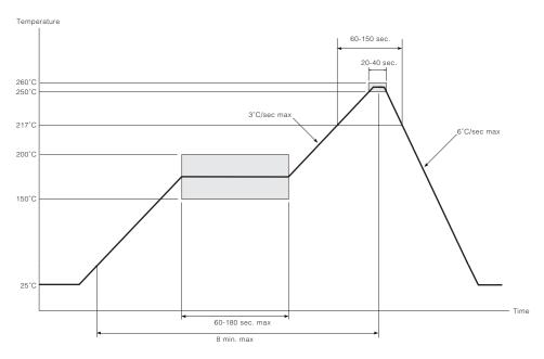
Figure 2-5: Maximum Pb-Free Solder Reflow Profile (Preferred)
