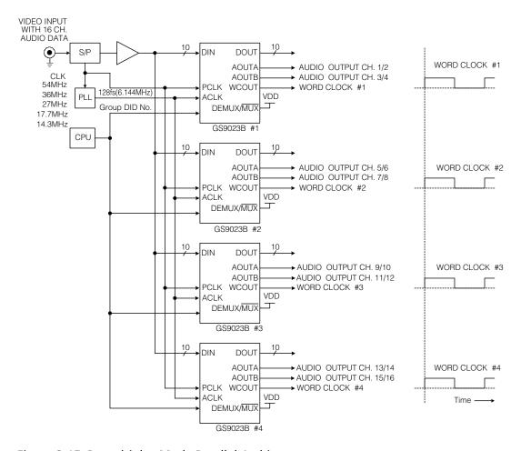
Figure 3-15: Demultiplex Mode Parallel Architecture
