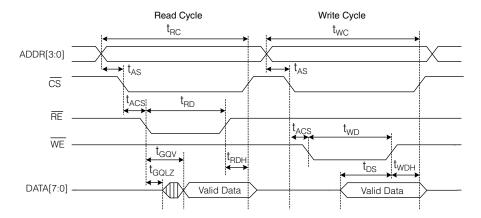
Figure 2-3: Host Interface Timing Diagram
