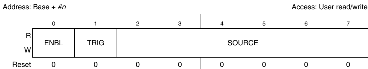
Figure 20-2. Channel Configuration Registers (CHCONFIG#n)
