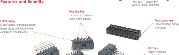
Choice of 3 throughhole soldertail lengths (2.60, 3.60 and 4.60mm) Supports different PCB thickness
