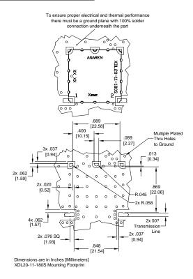
In order for Xinger surface mount delay lines to work optimally, there must be  $50\Omega$  transmission lines leading to and from all of the RF ports. Also, there must be a very good ground plane under the part with a number of plated thru holes to ensure proper electrical performance. If any of these conditions are not satisfied, insertion loss, average delay and VSWR may not meet published specifications.
