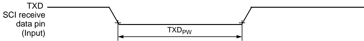
Figure 10-17 TXD Pulse Width
