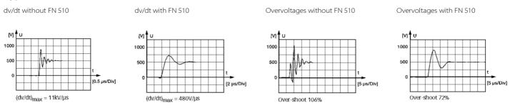
dv/dt reduction: maximum dv/dt at the motor terminals, measured with the motor drive operating at 14 kHz switching frequency, 5m of shielded cable, motor with 100% load. Overvoltage limitation: maximum overvoltages at the motor terminals, measured with the motor drive operating at 14 kHz switching frequency, 80 m of shielded cable, motor idling.
