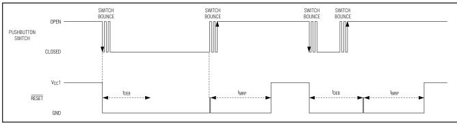
Figure 2. MAX6740/MAX6741/MAX6742 Manual Reset Timing Diagram
