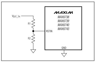
Figure 3. Monitoring an Additional Voltage
