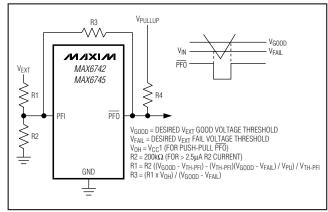
Figure 6. Adding Hysteresis to Power Fail for Push-Pull PFO
