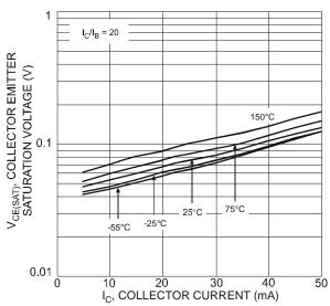
Fig. 3 Collector Emitter Saturation Voltage vs. Collector Current
