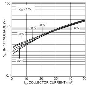
Fig. 4 Input Voltage vs. Collector Current
