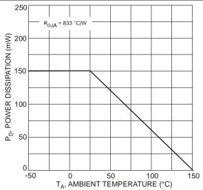
Fig. 1 Power Dissipation vs. Ambient Temeprature
