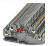
Disconnect terminal block, double level with angled contour and two disconnect points, Connection type: Pushin connection, Cross section: 0.14 mm<sup>2</sup> - 4 mm<sup>2</sup>, AWG: 26 - 12, Nominal current: 20 A, Nominal voltage: 400 V, Length: 127.5 mm, Width: 5.2 mm, Color: blue, Assembly: NS 35/7,5, NS 35/15
