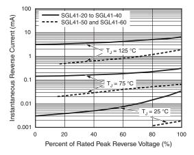
Fig. 4 - Typical Reverse Characteristics
