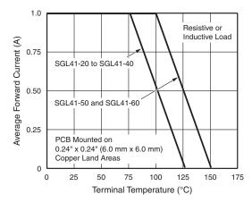
Fig. 1 - Forward Current Derating Curve
