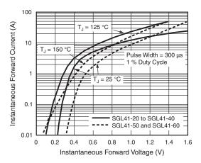
Fig. 3 - Typical Instantaneous Forward Characteristics
