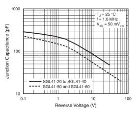
Fig. 5 - Typical Junction Capacitance
