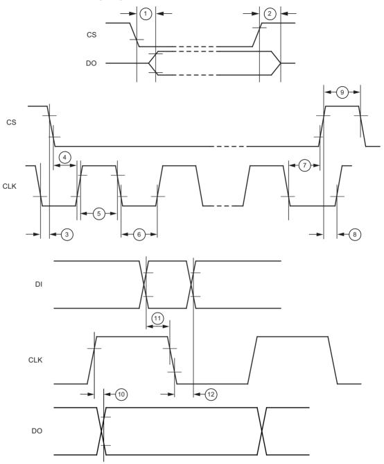
Inputs DI, CLK, CS: High level = 0.7 x V<sub>CC</sub>, low level = 0.3 x V<sub>CC</sub> Output DO: High level = 0.8 x V<sub>CC</sub>, low level = 0.2 x V<sub>CC</sub>
