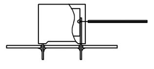
Temperature monitored inside the capacitor.
