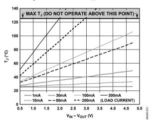
Figure 35. 0 mm<sup>2</sup> of PCB Copper,  $T_A = 25$ °C
