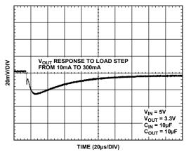
Figure 32. Output Transient Response,  $C_{OUT} = 10 \mu F$
