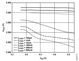
Figure 11. Output Voltage vs. Input Voltage
