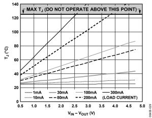
Figure 33. 500 mm<sup>2</sup> of PCB Copper,  $T_A = 25^{\circ}$ C
