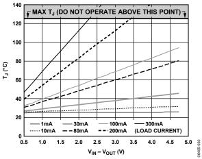
Figure 34. 100 mm<sup>2</sup> of PCB Copper,  $T_A = 25$ °C
