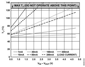
Figure 38. 0 mm<sup>2</sup> of PCB Copper,  $T_A = 50$ °C
