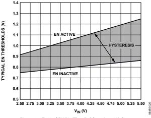
Figure 30. Typical EN Pin Thresholds vs. Input Voltage
