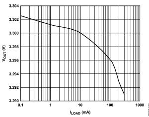
Figure 10. Output Voltage vs. Load Current
