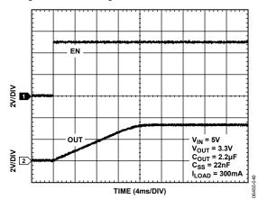
Figure 26. OUT Ramp-Up with External Soft-Start Capacitor
