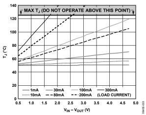
Figure 37. 100 mm<sup>2</sup> of PCB Copper,  $T_A = 50$ °C
