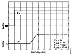
Figure 27. OUT Ramp-Up with Internal Soft-Start
