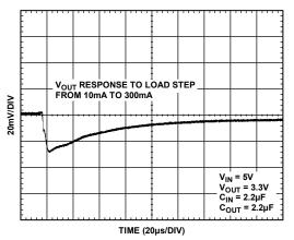
Figure 31. Output Transient Response,  $C_{OUT} = 2.2 \mu F$
