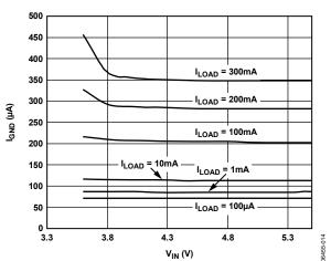
Figure 14. Ground Current vs. Input Voltage
