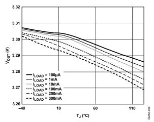
Figure 9. Output Voltage vs. Junction Temperature
