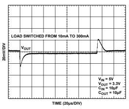
Figure 19. Load Transient Response
