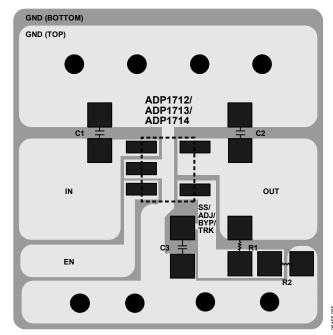
Figure 39. Example PCB Layout
