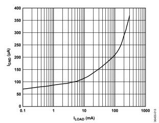
Figure 13. Ground Current vs. Load Current
