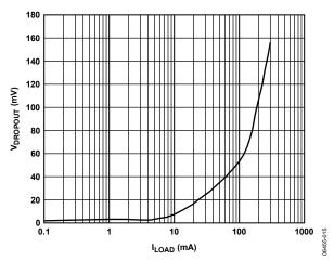
Figure 15. Dropout Voltage vs. Load Current
