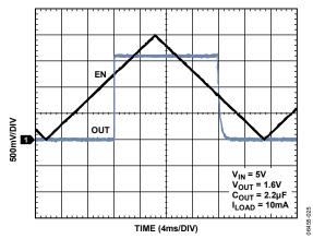
Figure 29. ADP1712 Adjustable Typical EN Pin Operation
