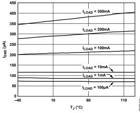
Figure 12. Ground Current vs. Junction Temperature
