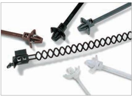
A wide range of arrowhead fixing ties which are suitable for panel thicknesses of 0.5mm to 4.5mm and hole diameters of 4.4mm to 8.0mm.
