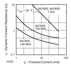
Fig. 2 - Dynamic Forward Resistance vs. Forward Current
